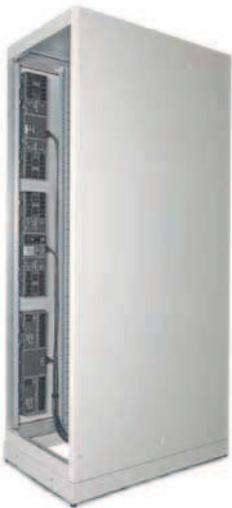
*All DI-STRIP HighPower are equipped with especially flat housing extrusions and side cable entry. This enables installation without any loss of usable height units and cable entry from above and below. Full accessibility to the 19" level with 600 mm wide server racks is also a given.*
