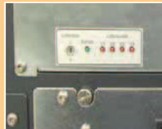
Fan failure display/ four speed levels
